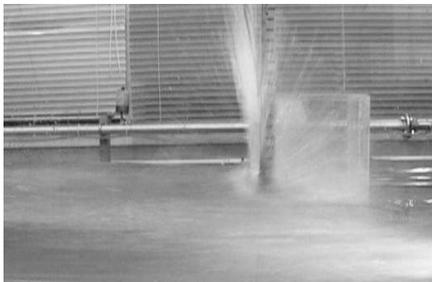
Moment of the impact of tsunami and the splash of water
