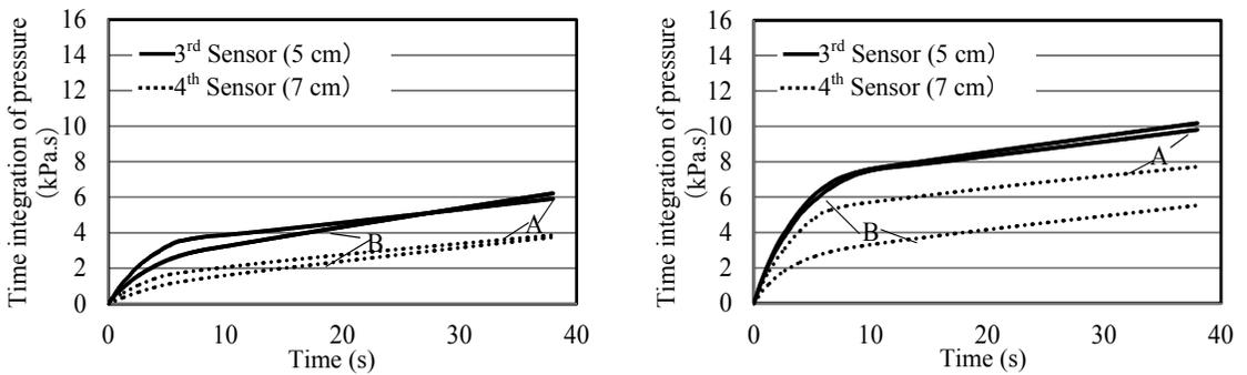
Fig.7 Time integration of impact pressure for impoundment depths of 20 cm (left) and 30 cm (right) on the 3<sup>rd</sup> and 4<sup>th</sup> sensors (A: model A, B: model B).
