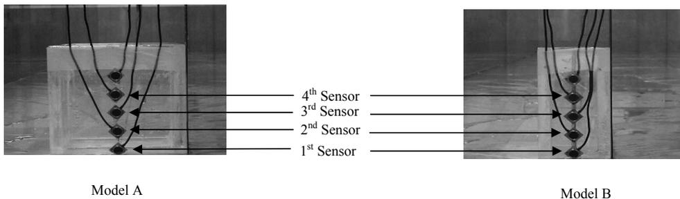
**Fig.2** Building models with pressure sensors.
