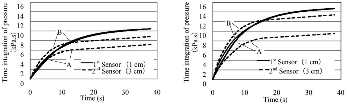
Fig.6 Time integration of impact pressure for impoundment depths of 20 cm (left) and 30 cm (right) on the 1<sup>st</sup> and 2<sup>nd</sup> sensors (A: model A, B: model B).
