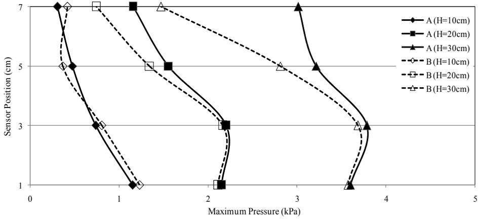
Fig.5 Maximum pressure distribution (A: model A, B: model B).
