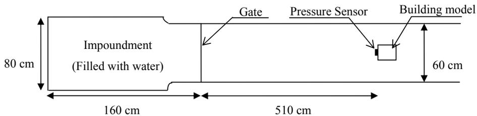
**Fig.1** Experimental channel with building model: plan view.
