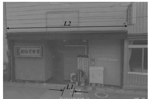
Fig.4 The estimation of the building width of the point No. 10 from the Google Street View.
