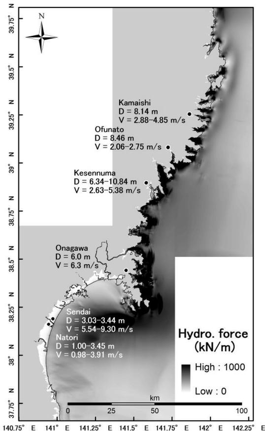
Fig.3 Simulated hydrodynamic force and estimated flow velocity in 150\*150 m<sup>2</sup> grid
