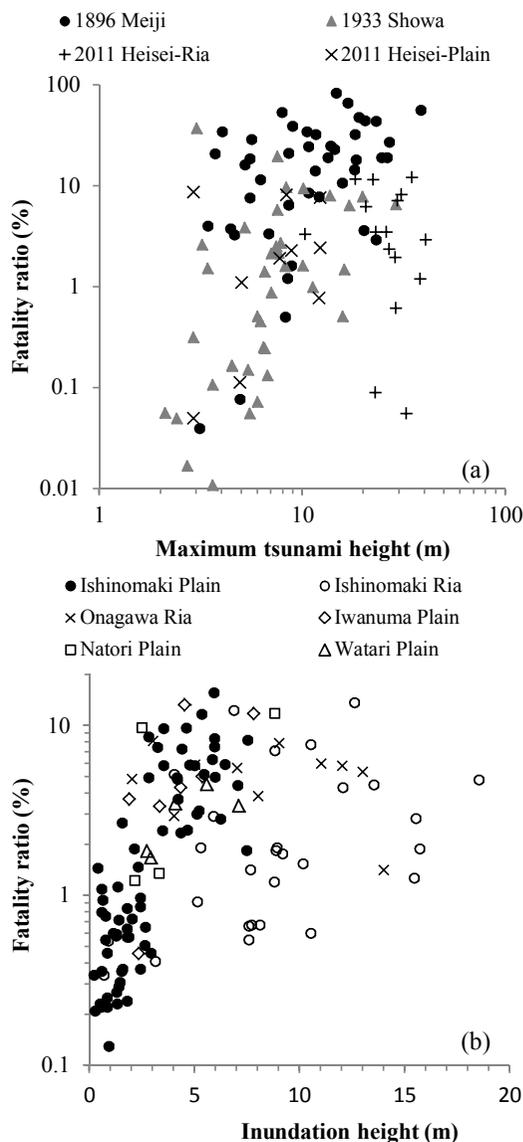
**Fig.1** Tsunami fatality ratio in Tohoku region from (a) Historical tsunamis in Sanriku and (b) the 2011 tsunami
