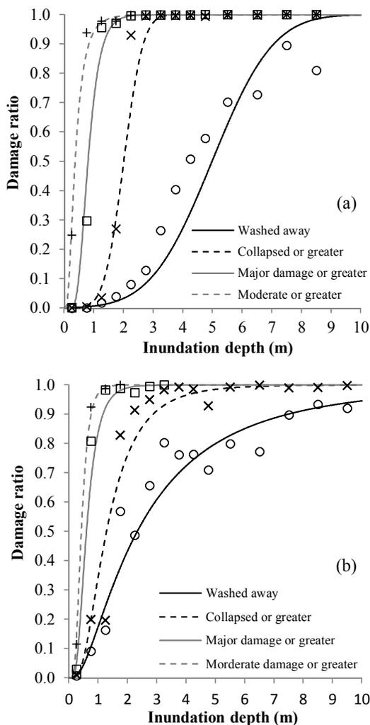
**Fig.2** Vulnerability curves developed from damaged buildings in Ishinomaki city in (a) Plain coasts and (b) Ria coasts
