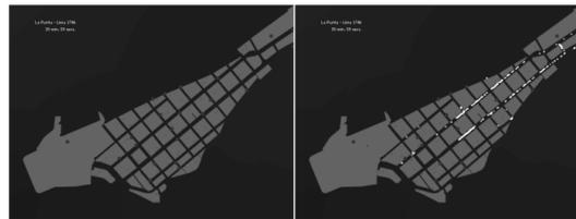
**Fig.9** Snapshot at 40min simulation for the Vertical Evacuation case (left) and the Horizontal and Vertical Evacuation case (right). White dots show areas of stagnation.
