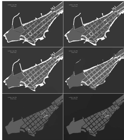
**Fig.8** Horizontal Evacuation Case. Casualties are observed at traffic congestion near the exit of the district. The necessity of a vertical evacuation is revealed here.
