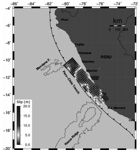
**Fig.3** Slip distribution from GPS data. There are 280 sub-faults of 20x20km. (Pulido et.al, 2011) (Figure in Yauri, S. (2011)).
