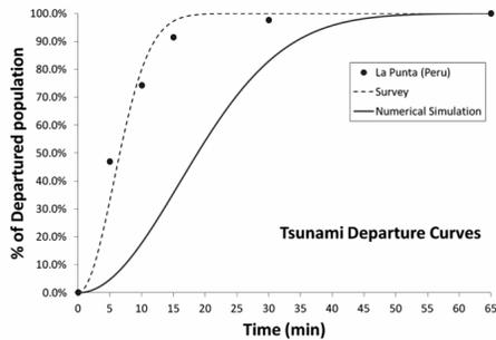
**Fig.7** Tsunami Departure Curves for the simulation cases. Behavior of start time is obtained through the stochastic simulation of random selected times bounded by two Rayleigh distributions. Left distribution obtained through stated preference surveys and the other distribution is based on the estimated arrival time of tsunami from numerical simulation.
